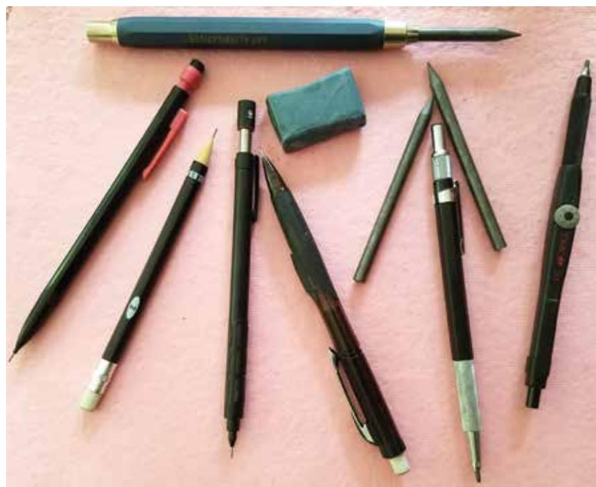
An assortment of some of the many mechanical pencils available today. At left is a disposable, non-refillable pencil. At center are several refillable, click-style pencils with features including removable erasers, storage areas for extra lead, and soft, comfortable grips. At right and at top are claw-style holders, with features including built-in sharpeners and grade-indicator wheels.
